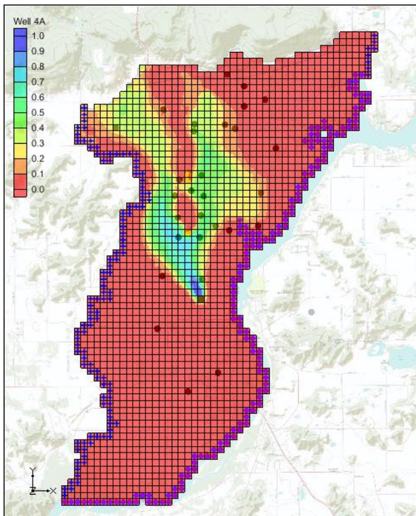
Figure 9 Probabilistic capture zone for proposed well
