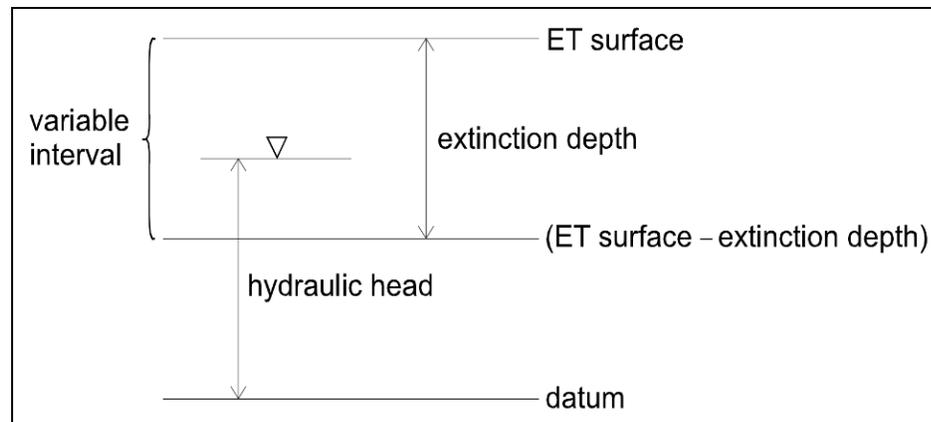
Figure 1 ET model, from Banta, 2000<sup>1</sup>
